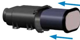
**6 Insert the primary filter.** For PSD08, slide the filter into the housing until the gasket seats against the housing. For PSD09, 10 and 12, slide the filter down at a 5° angle until it hits the end of the housing. Push the filter toward the outlet section to complete the seal.
