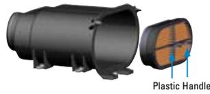
**5 If replacing safety,** using the plastic handle on the safety filter, slide the filter at an angle into the outlet side and push in place until the filter seats firmly and evenly within the housing. *Note: On PSD10 and 12 models, insert the safety filter tab into the positioning slot before pushing the filter in place.*
