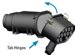
**7 Replace the service cover.** On PSD08, insert the hinge tabs into the housing and tilt up the service cover up and secure latches. For the PSD09, 10, 12, placed the service cover in position and fasten the latches. *Note: If the cover doesn't seat, remove and re-check the filter position. Cover will be difficult to install if filter isn't installed correctly.*
